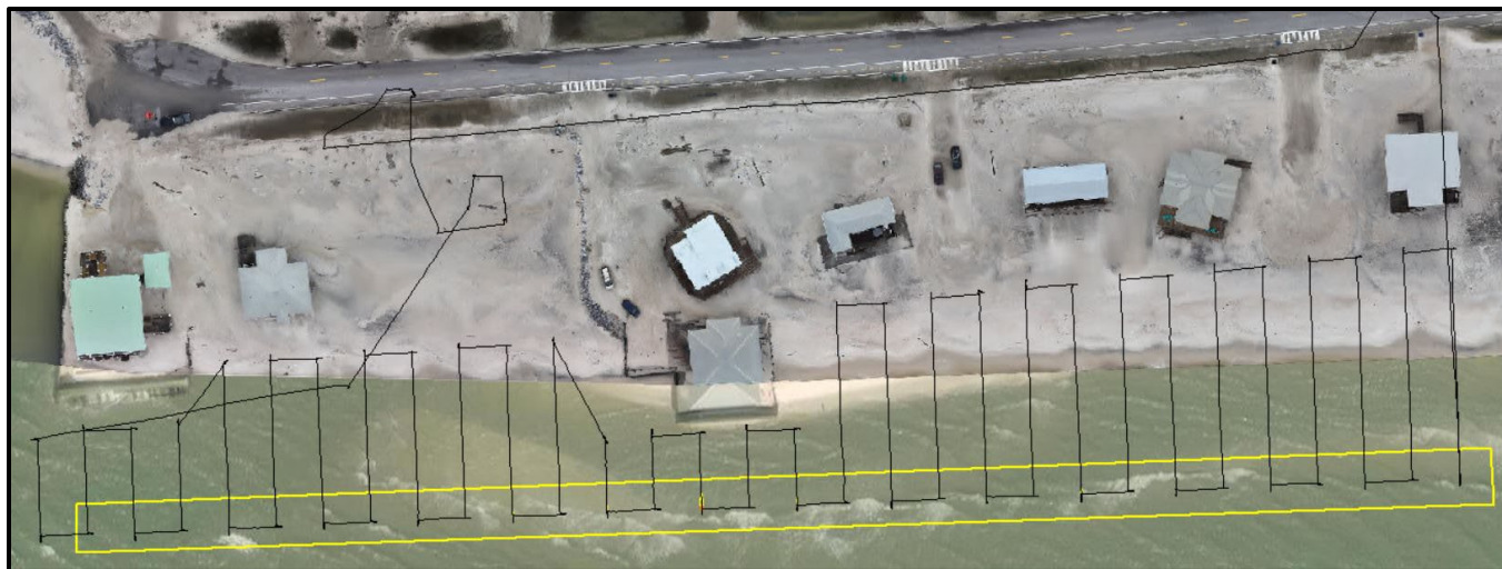
Figure 30. Aerial view showing transect coverage with highlighted area for further analysis. Small hits in the data at the end of the transects are an artifact of the drone repositioning and turning the sensor in the magnetic field.
