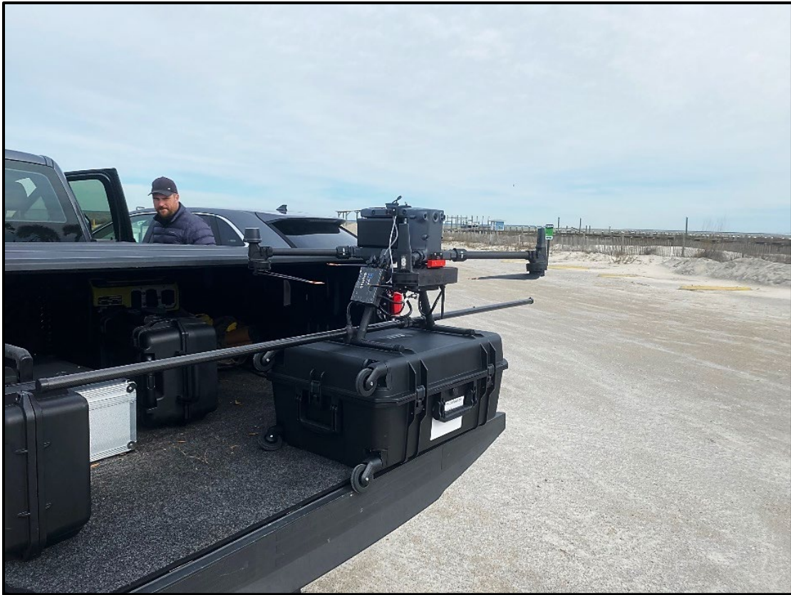
Figure 23. Assembled MagDroneR4, pre-launch.
